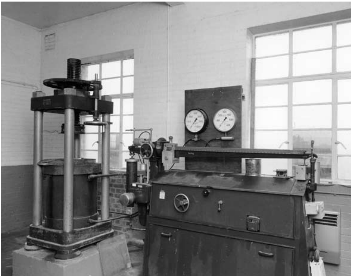
Figure 29: Office, Casting Workshop and Laboratory S5, press by A Macklow Smith Ltd, London and a Beacham high pressure oil pump. These were used for stress testing various materials. (c) English Heritage BB99/15969
