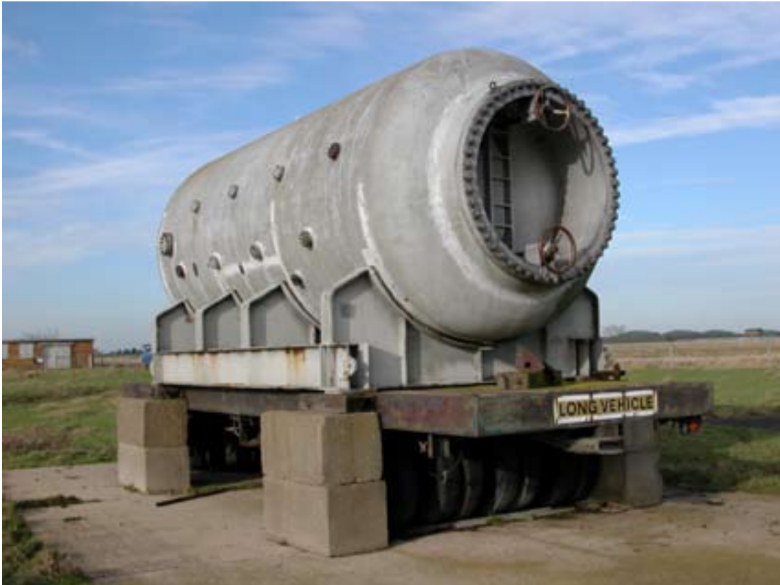
Figure 27: Pressure Vessel EHK, within this vessel by reducing the pressure scientists could simulate high altitude conditions. (c) English Heritage
